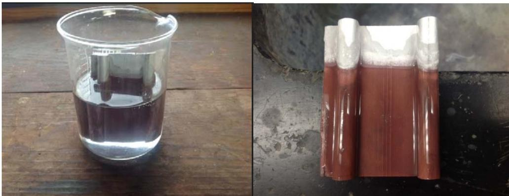
To prevent re-contamination of the electrolyte, we suggest bagging the cathode to prevent this material from sluffing off and begin to circulate in the electrolyte.
