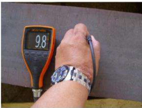
Mill scale with 80% magnetite ( \text{FeO} \cdot \text{Fe}_2\text{O}_3 ), thickness is 9.8 microns.
